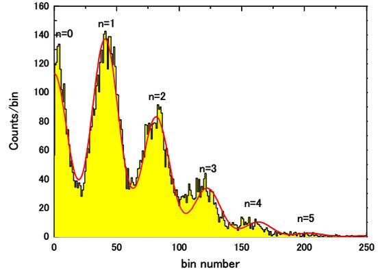
Figure 3: Pulse height spectrum from the Ti-TES in response to 1550 nm photon pulses.
