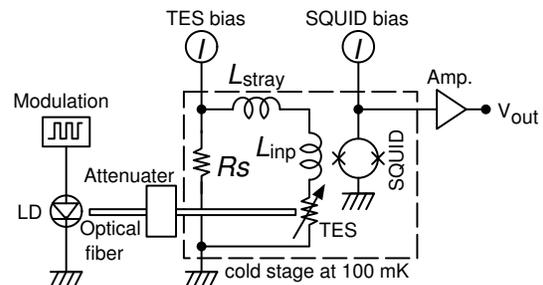
Figure 1: The experimental setup for photon number measurements
