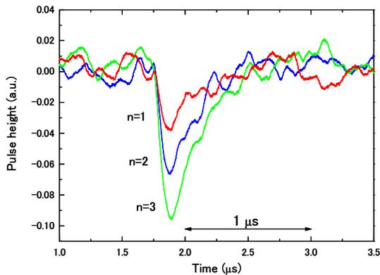
Figure 2: The examples of photon measurement signals with the Ti-TES.
